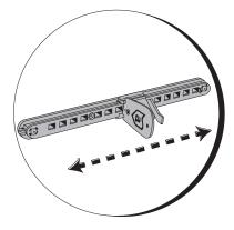
The adjustment lever can be pulled toward you with the opposite foot to create hands-free adjustment, if necessary.
